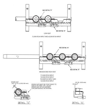
Fig. 35 - Spark Adjustment (04-07)
